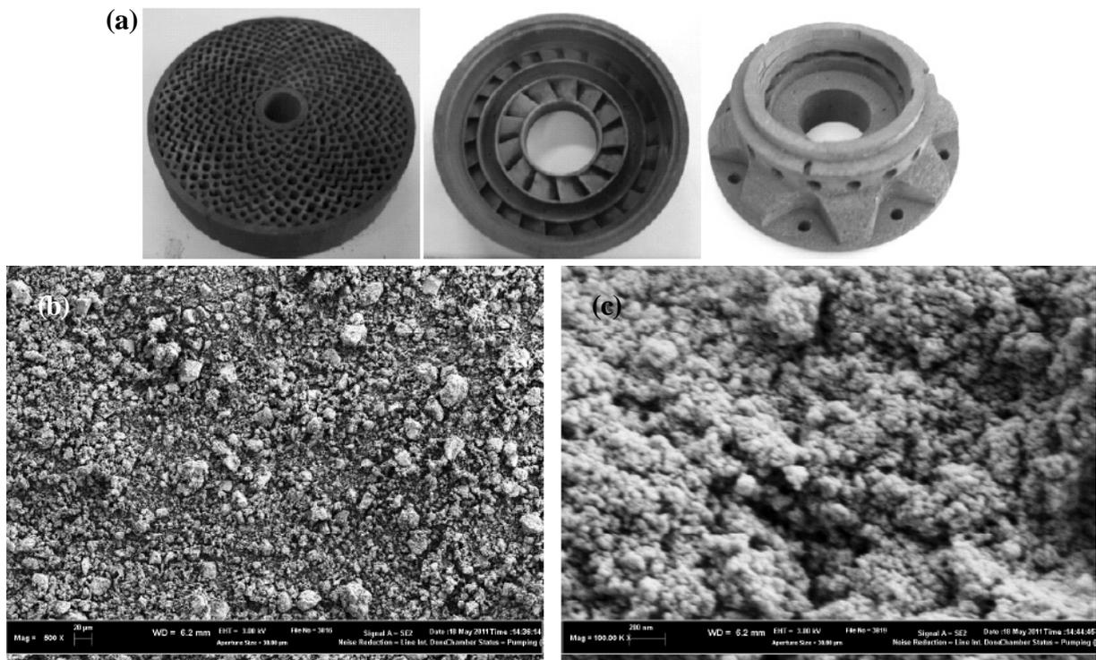
**Fig. 1.** (a) Photos of the parts of ceramic microturbine manufactured by AT, typical linear dimensions of the units are 3-5 cm; (b) SEM data on ceramics microstructure. Reprinted with permission from J. Timonen, M. Mylly, V. G. Konakov, A. V. Soudarev and I. Yu. Archakov, Structure of a ceramic material developed by laser prototyping techniques, *Reviews on Advanced Materials Science* vol 29 (2011) pp 175-179.
