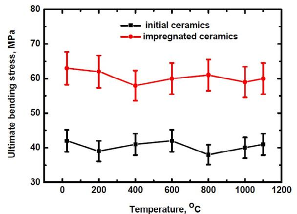
**Fig. 5.** Impregnation results: the comparison of ultimate bending stress for the initial ceramics and the same materials after 4 impregnation cycles, the accuracy of the measurements was  $\pm 10\%$ .
