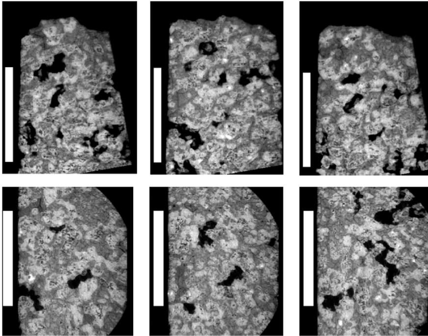
**Fig. 2.** Material porosity characterization according to X-ray tomography data (Xradia MicroCT-400,  $E_{\max} = 40$  keV): upper line – “side-to-side” scanning, bottom line “top – down” scanning; the scale bar is 500  $\mu\text{m}$ .
