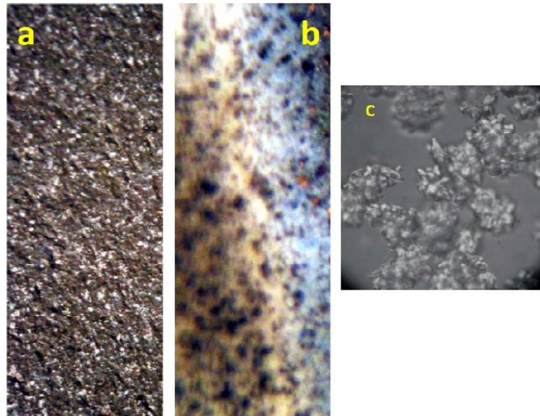
**Fig. 3.** The photo of the ceramic unit wall surface (optical microscopy at x125): (a) before impregnation and (b) after impregnation; (c) cordierite structure grown in the materials pores.
