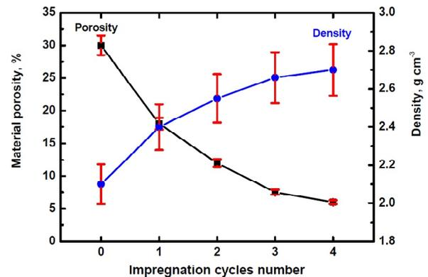
**Fig. 4.** Impregnation results: the changes in materials porosity and ceramics density (measurements accuracy 7%).
